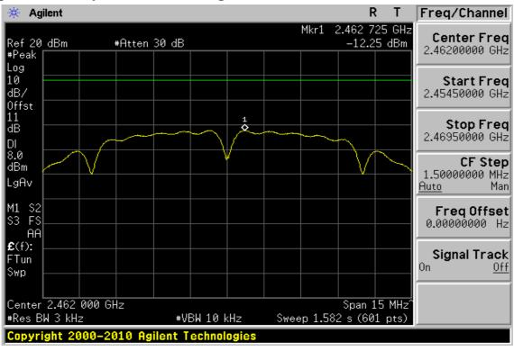
802.11g **Power Spectral Density Test Plot (CH-Low)**
