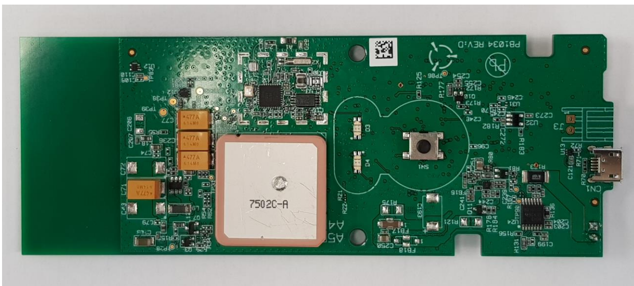
Fig. 10 PC Board Back View with BLE Circuitry Cover Removed
