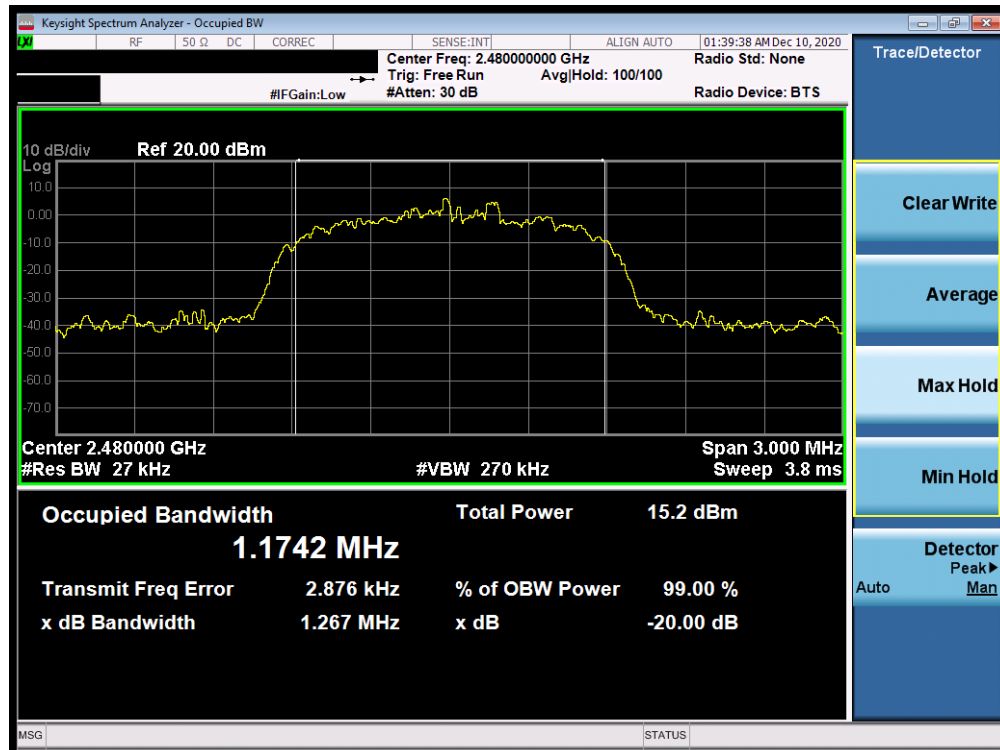
Plot 7-9. 20dB Bandwidth Plot (Bluetooth, 3Mbps – Ch. 78)
