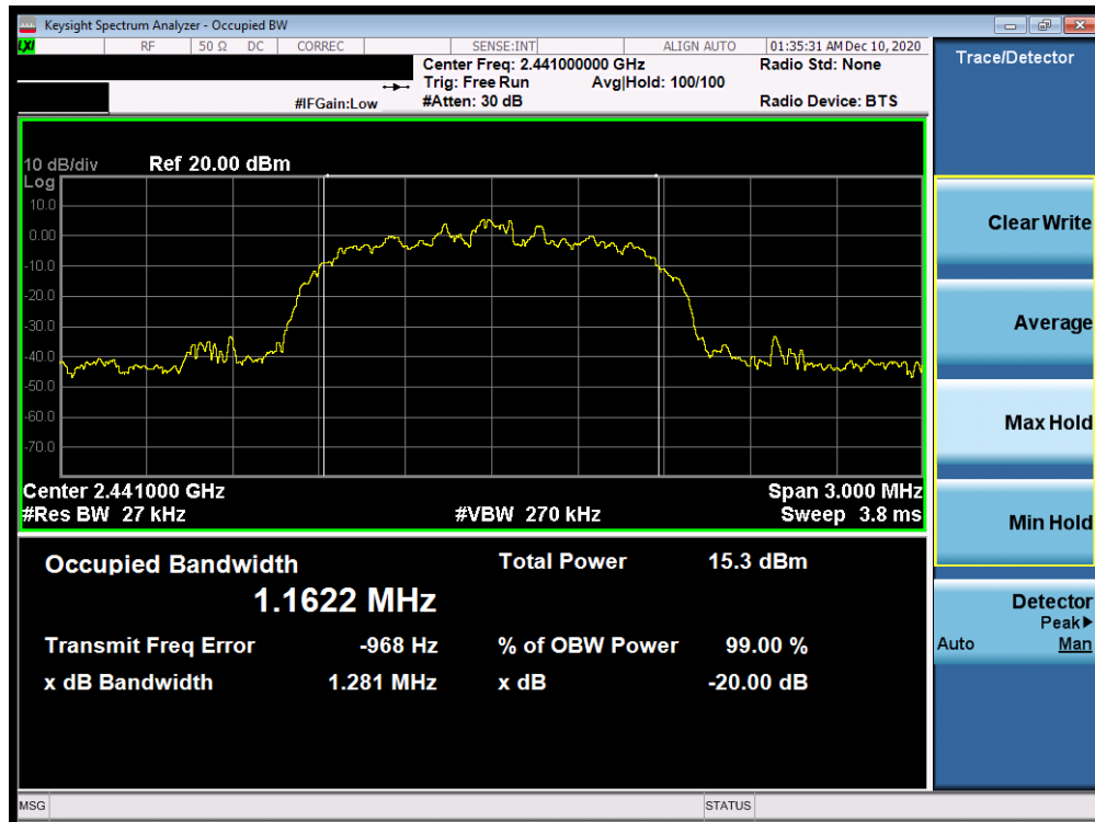
Plot 7-5. 20dB Bandwidth Plot (Bluetooth, 2Mbps – Ch. 39)
