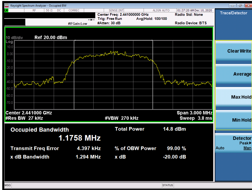
Plot 7-8. 20dB Bandwidth Plot (Bluetooth, 3Mbps – Ch. 39)
