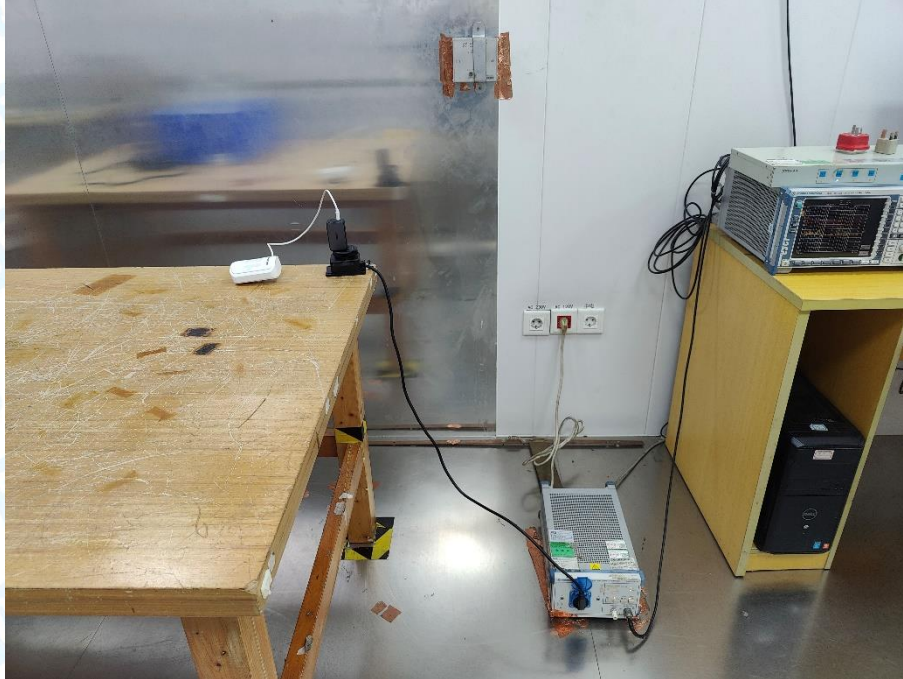
Photo of Setup for Radiated Emission (30MHz~1GHz)
