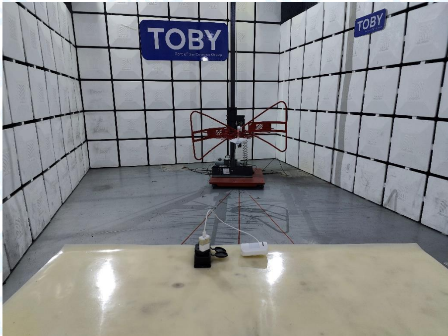
Photo of Setup for Radiated Emission (30MHz~1GHz)
