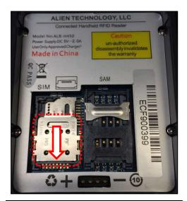
Locate the SIM card holder and **SLIDE** it downward to release it.
