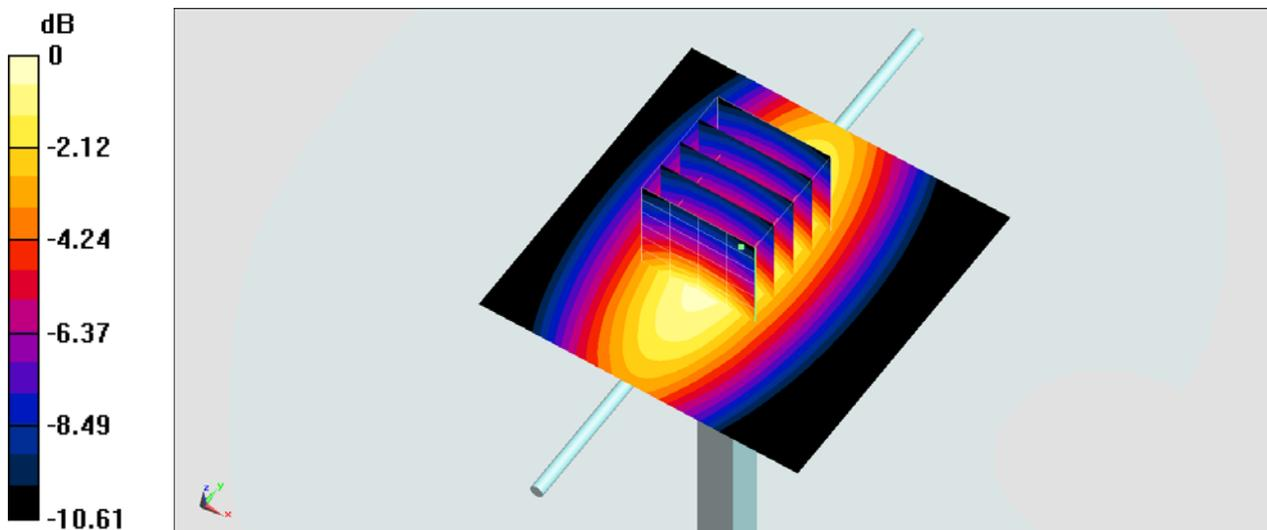
0 dB =  $3.27 \text{ W/kg} = 5.15 \text{ dBW/kg}$
