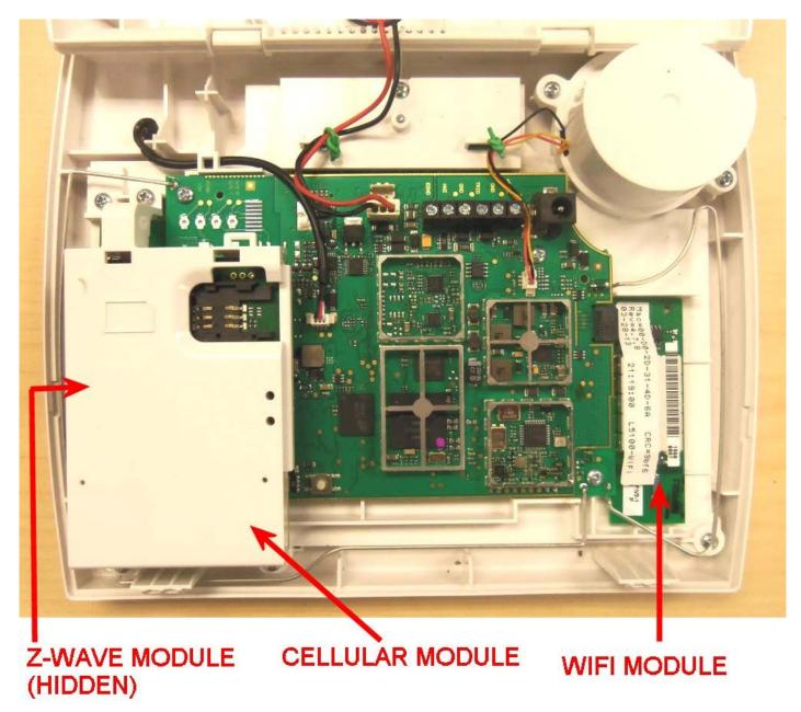
FOR REFERENCE: CASE OPEN, CLOSE UP, Z-WAVE, WIFI, AND CELL MODULES INSTALLED:
