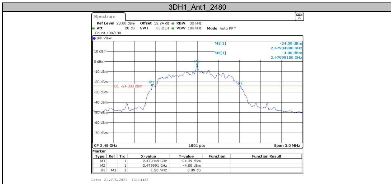
**Appendix B: Occupied Channel Bandwidth****Test Result**
