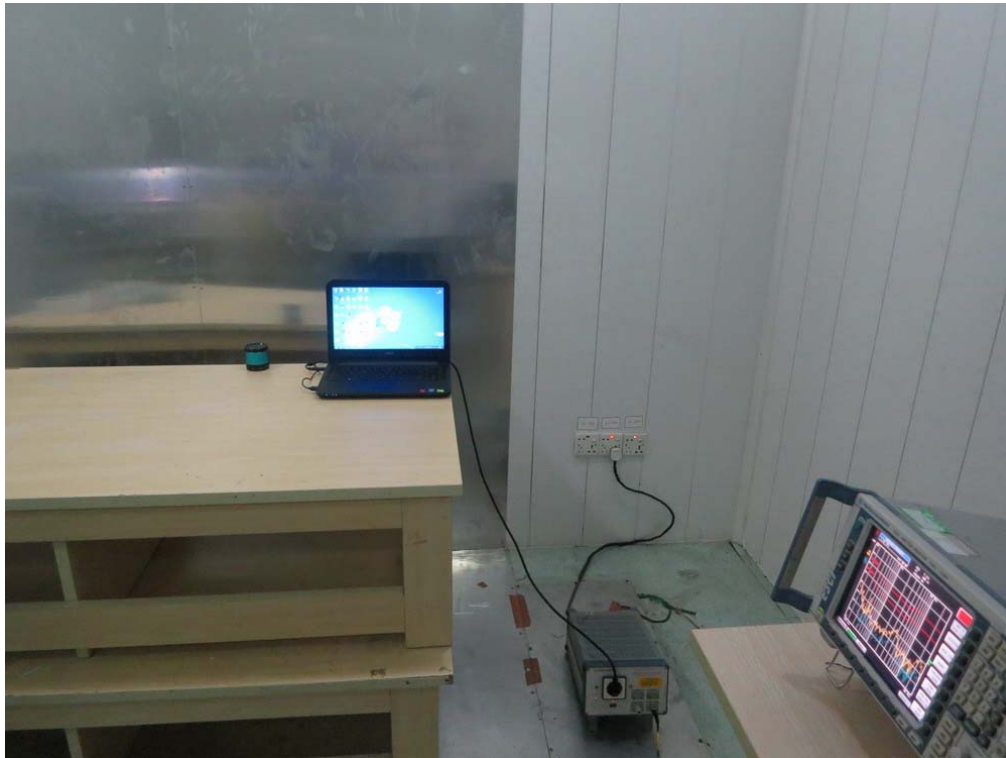
FCC RADIATED EMISSION TEST SETUP
