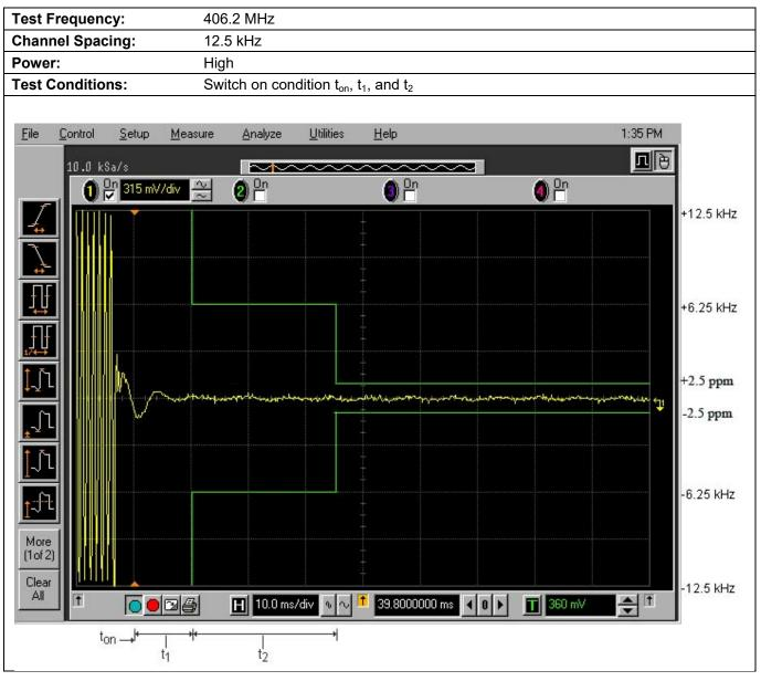
Plot 5.12.3.4. Transient Frequency Behavior for 12.5 kHz Channel Spacing
