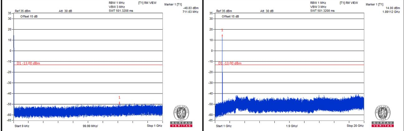
Note: The signal over the limit in 9 kHz is from spectrum analyzer.
