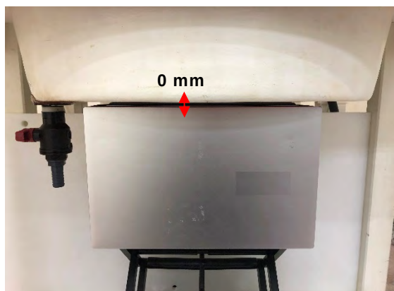
Fig.3 EUT Bottom side to flat phantom
