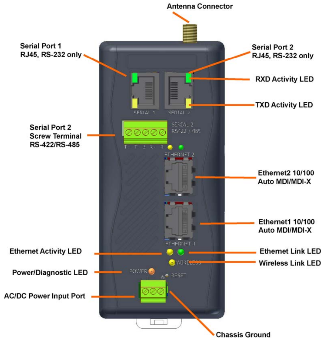
Figure 4-6. XPress DR+W Front Panel Layout
