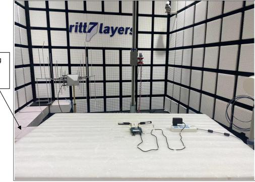
the absorbing material is under the foam
