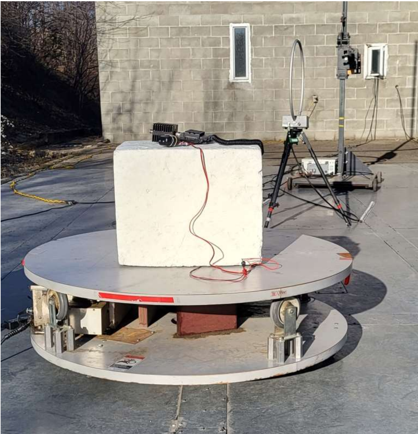
Figure E11.2 – Setup, Radiated Measurements, 9kHz – 30MHz, Without Accessories
