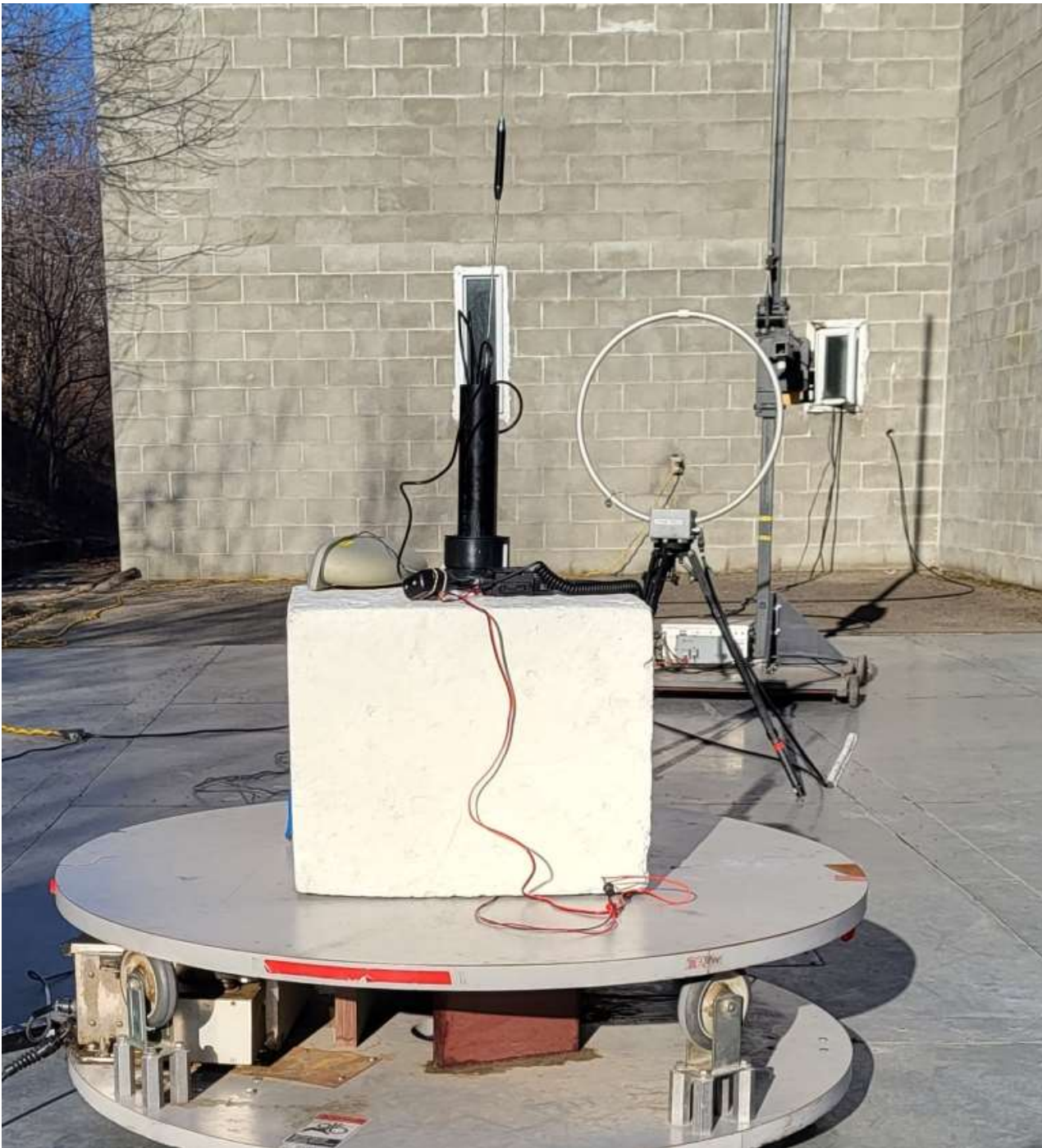
Figure E11.3 – Setup, Radiated Measurements, 9kHz – 30MHz, With Accessories
