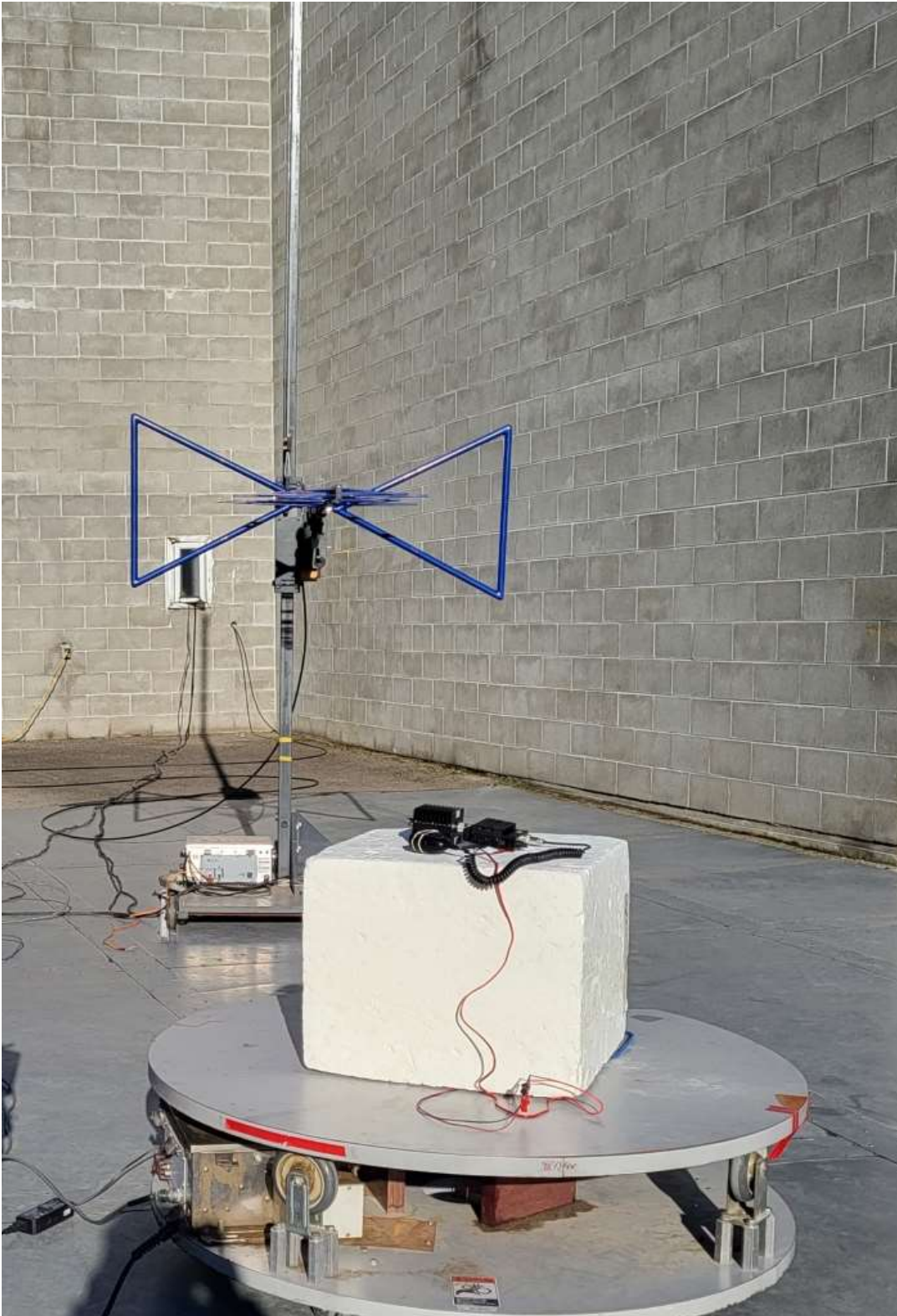
Figure E11.4 – Setup, Radiated Measurements, 30 – 1000MHz, Without Accessories
