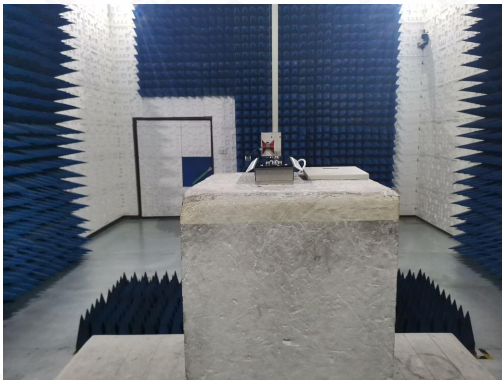
FCC RADIATED EMISSION TEST SETUP ABOVE 1GHZ
