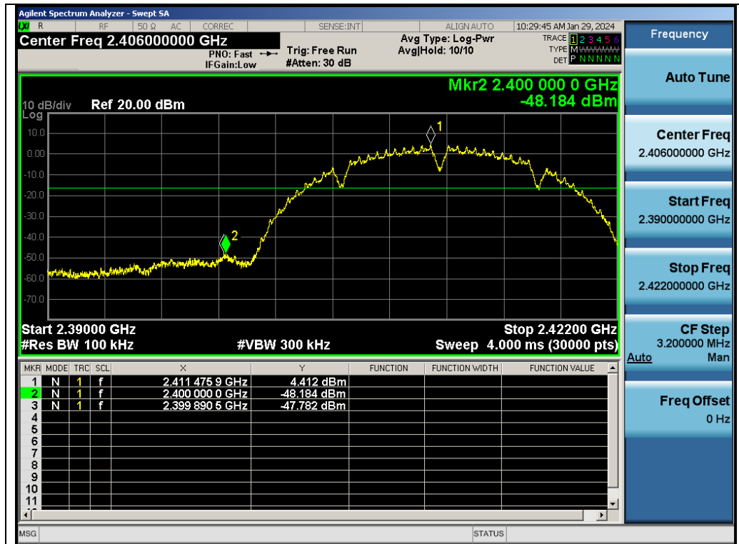
Test_Graph_802.11b_ANT1_2412_1Mbps_Lower Band Edge Emissions
