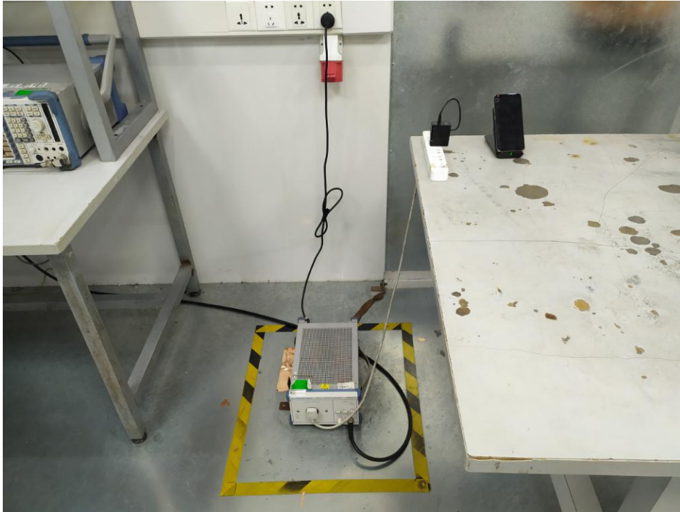
Photo of Conducted Emission Measurement
