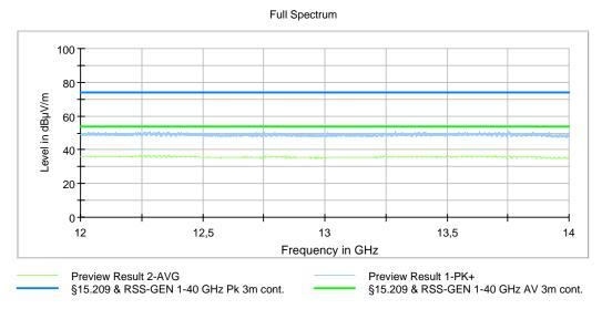
The results of the standard subsequent measurement above 1 GHz in a semi-anechoic chamber are indicated in the table below. The limits as well as the measured results (levels) refer to the above-mentioned standard while taking account of the specified requirements for a 3 m measuring distance.
