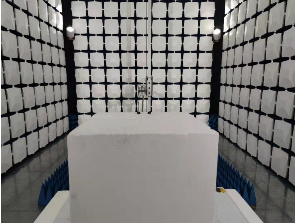
Above 1GHz for radiated emission test setup
