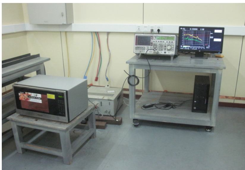
Conducted Emission Test Set-up
