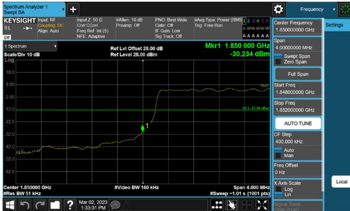
Sub6 n2. Lower Band Edge Plot (5 M BW Ch.370500 BPSK_RB25_Offset 0) -2
