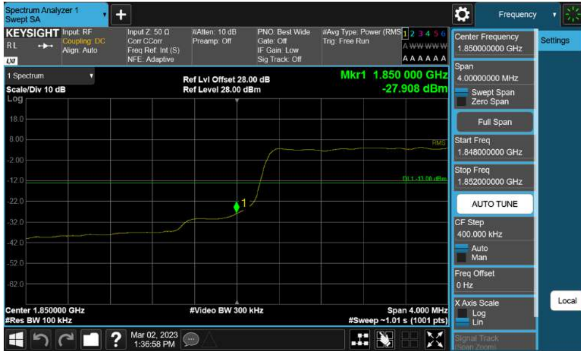
Sub6 n2. Lower Band Edge Plot (10 M BW Ch.371000 BPSK_RB50_Offset 0) -2
