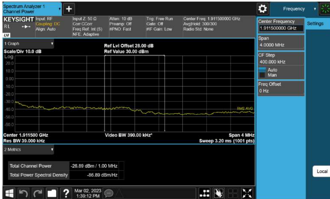
Sub6 n2. Upper Extended Band Edge Plot (10 M BW Ch.381000 BPSK_RB50_0) -3
