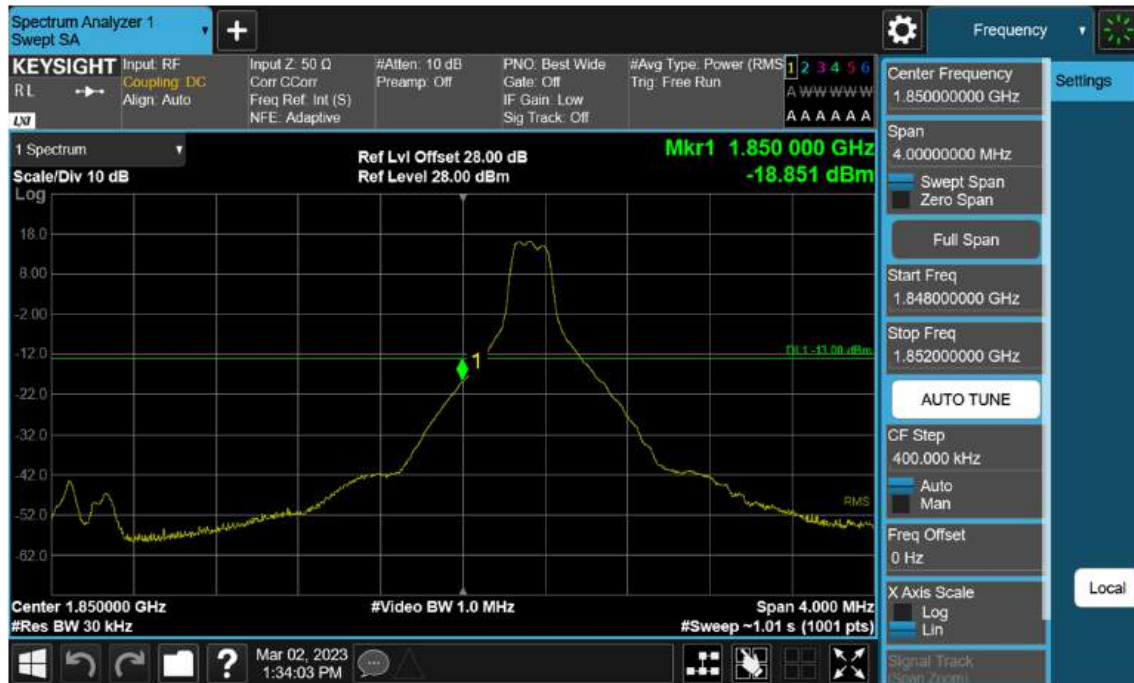
Sub6 n2. Lower Band Edge Plot (5 M BW Ch.370500 BPSK_RB1_Offset 0) -1
