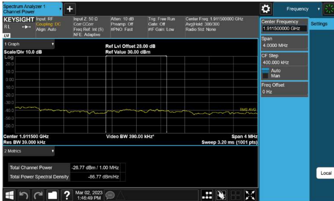
Sub6 n2. Upper Extended Band Edge Plot (20 M BW Ch.380000 BPSK_RB100_0) -3
