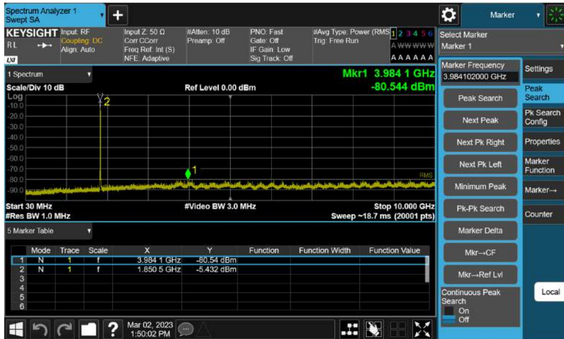
Sub6 n2. Conducted Spurious_1 (370500ch_5 MHz_BPSK_RB 1_1)
