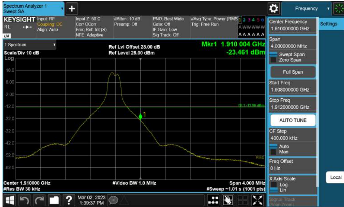
Sub6 n2. Upper Band Edge Plot (10 M BW Ch.381000 BPSK_RB1_Offset 51) -1
