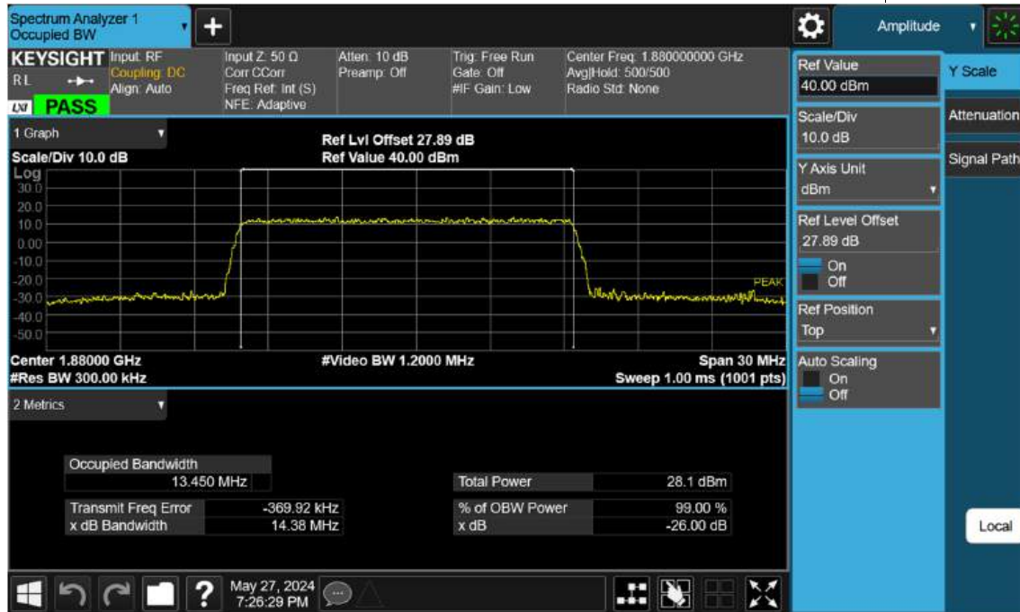
Sub6 n2. Occupied Bandwidth Plot (15 M BW Ch.376000 256QAM RB 75_0)
