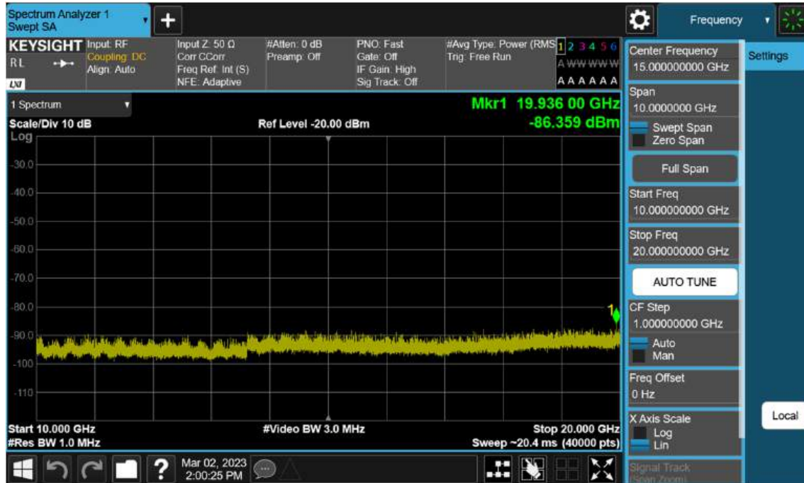
Sub6 n2. Conducted Spurious_2 (371500ch_15 MHz_ BPSK_RB 1_1)
