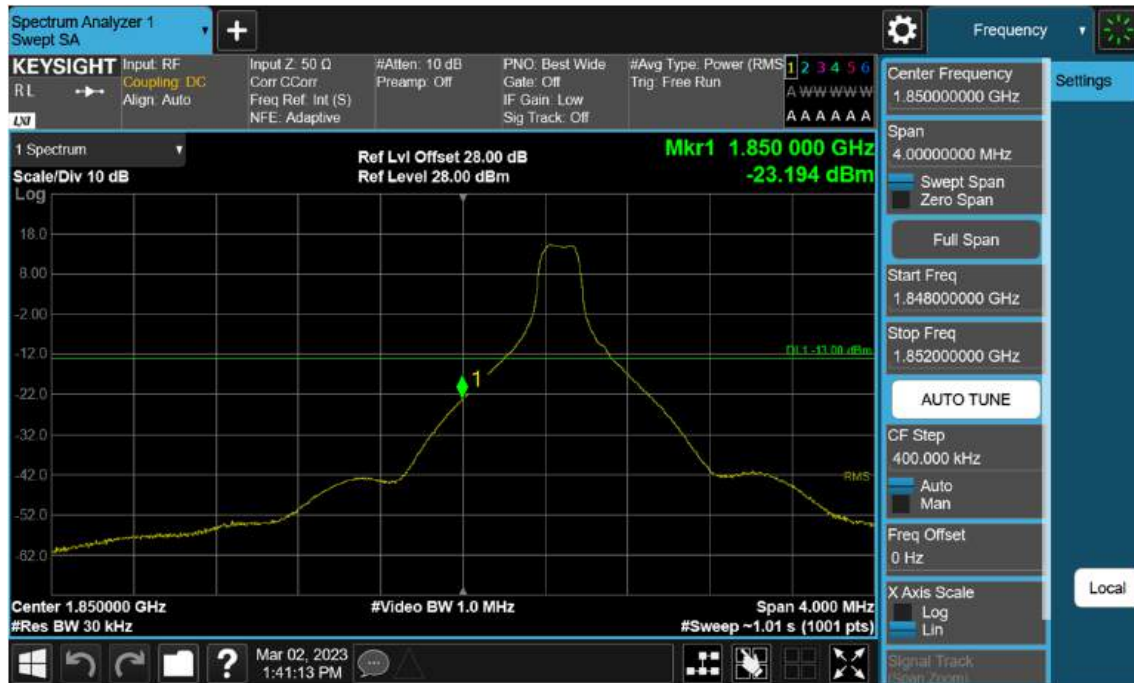
Sub6 n2. Lower Band Edge Plot (15 M BW Ch.371500 BPSK_RB1_Offset 0) -1
