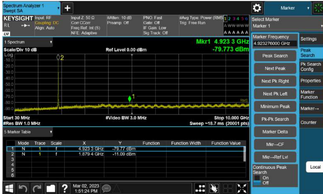
Sub6 n2. Conducted Spurious_1 (376000ch_5 MHz_BPSK_RB 1_1)
