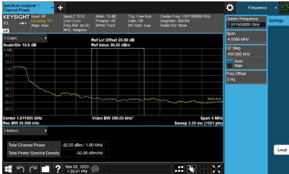
Sub6 n2. Upper Extended Band Edge Plot (5 M BW Ch.381500 BPSK_RB25_0) -3
