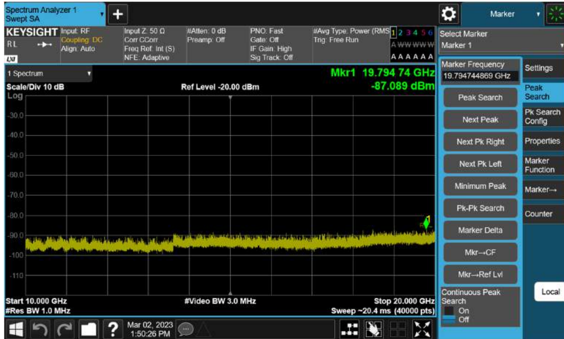
Sub6 n2. Conducted Spurious_2 (370500ch_5 MHz_BPSK_RB 1_1)
