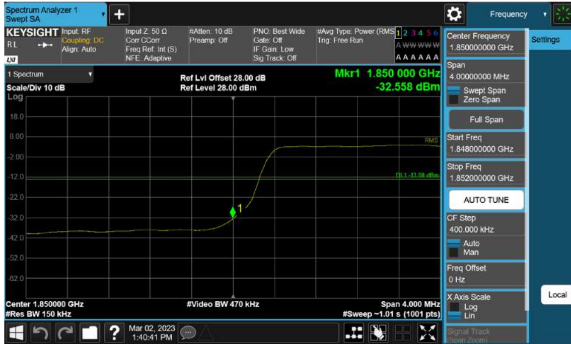
Sub6 n2. Lower Band Edge Plot (15 M BW Ch.371500 BPSK_RB75_Offset 0) -2
