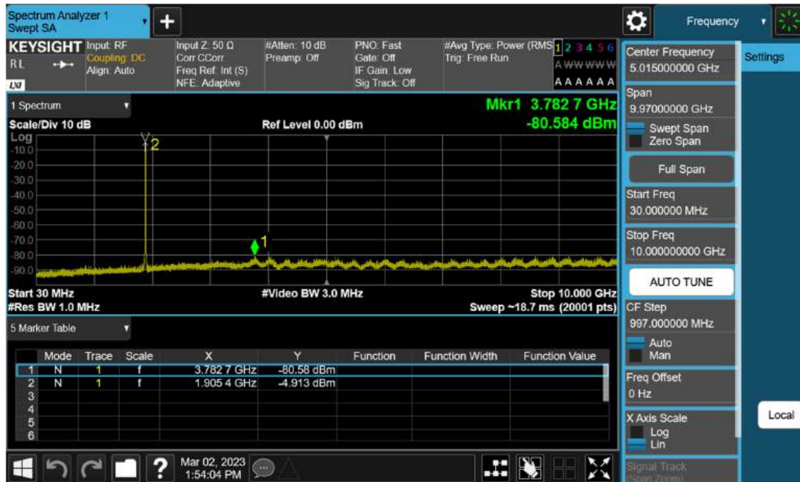
Sub6 n2. Conducted Spurious_1 (381500ch_5 MHz_ BPSK_RB 1_1)
