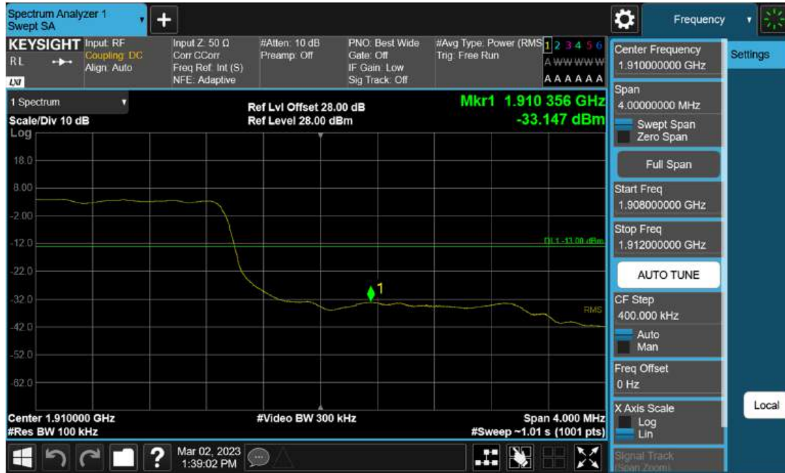
Sub6 n2. Upper Band Edge Plot (10 M BW Ch.381000 BPSK_RB50_Offset 0) -2
