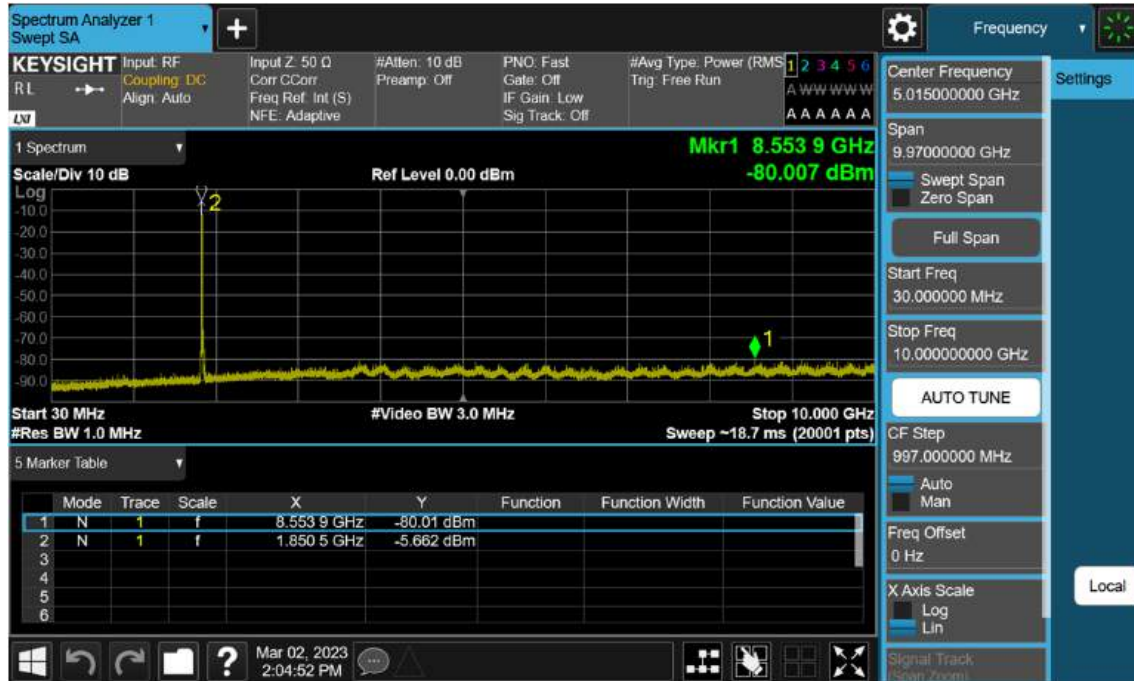
Sub6 n2. Conducted Spurious_1 (372000ch_20 MHz_ BPSK_RB 1_1)
