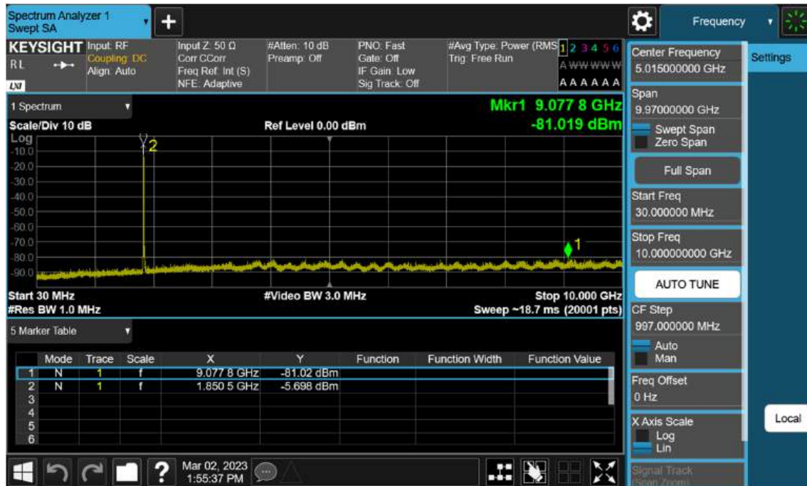
Sub6 n2. Conducted Spurious_1 (371000ch_10 MHz_ BPSK _RB 1_1)
