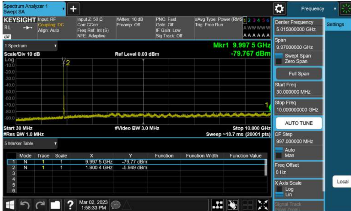
Sub6 n2. Conducted Spurious_1 (381000ch_10 MHz_ BPSK_RB 1_1)
