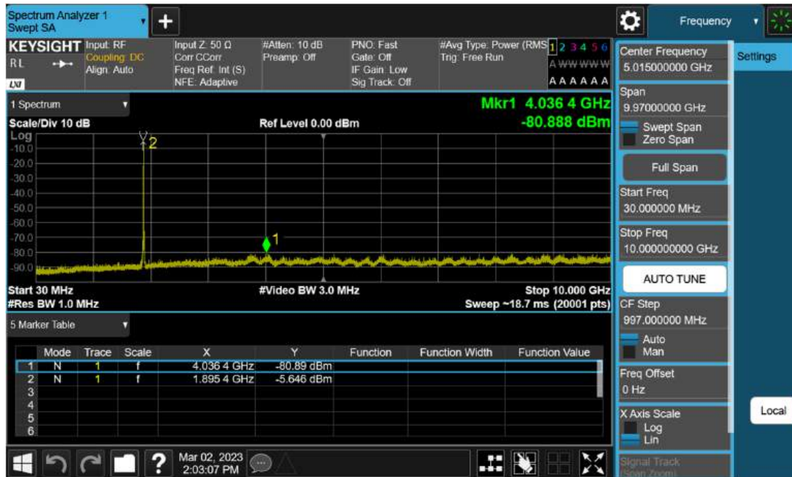
Sub6 n2. Conducted Spurious_1 (380500ch_15 MHz_ BPSK_RB 1_1)
