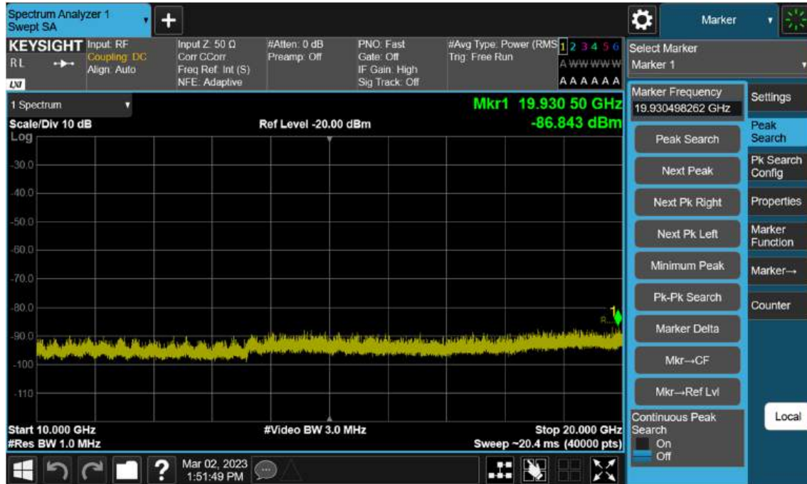
Sub6 n2. Conducted Spurious_2 (376000ch_5 MHz_ BPSK_RB 1_1)
