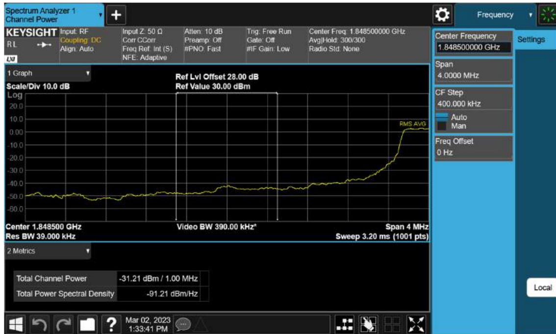
Sub6 n2. Lower Extended Band Edge Plot (5 M BW Ch.370500 BPSK_RB25_0) -3
