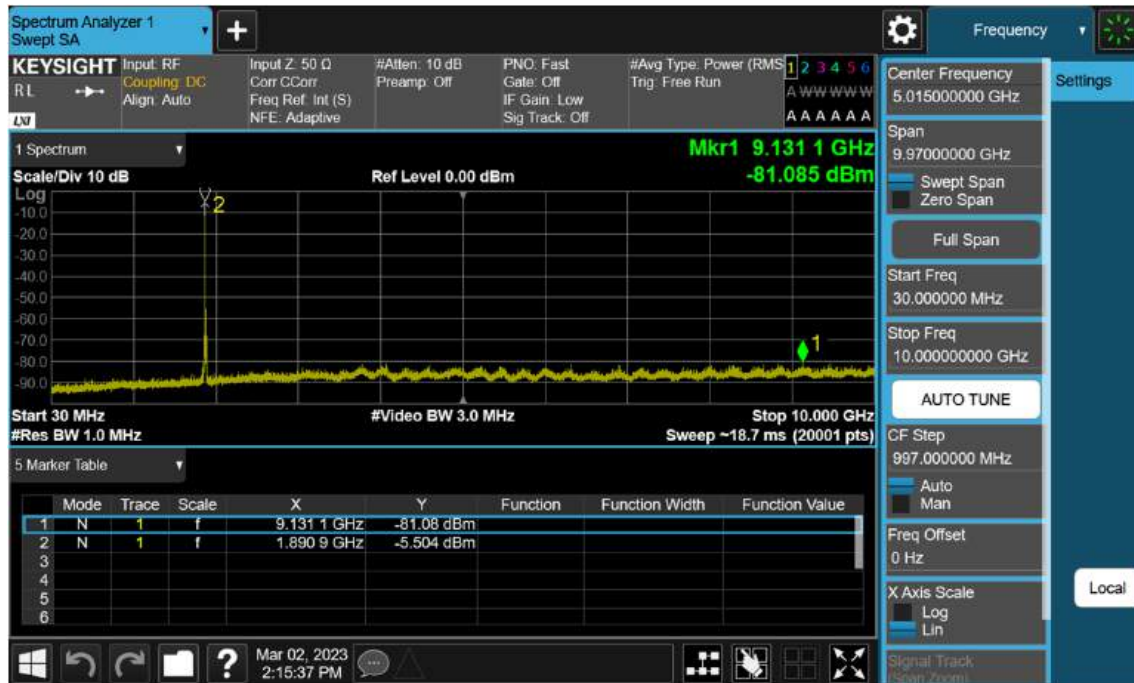
Sub6 n2. Conducted Spurious_1 (380000ch_20 MHz_ BPSK_RB 1_1)
