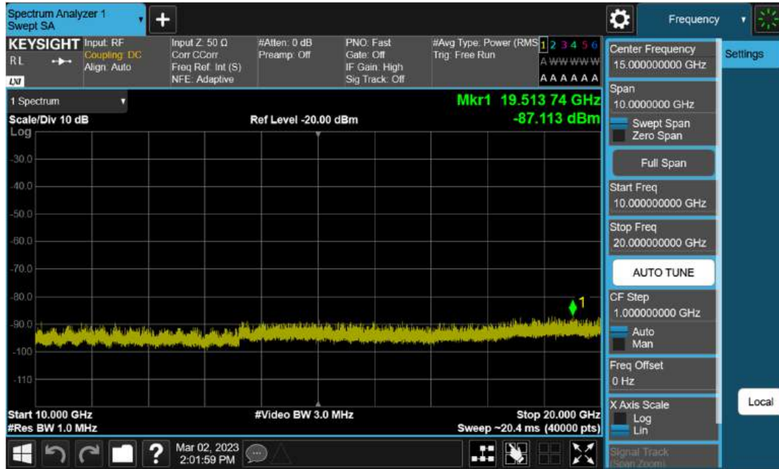
Sub6 n2. Conducted Spurious_2 (376000ch_15 MHz_ BPSK_RB 1_1)
