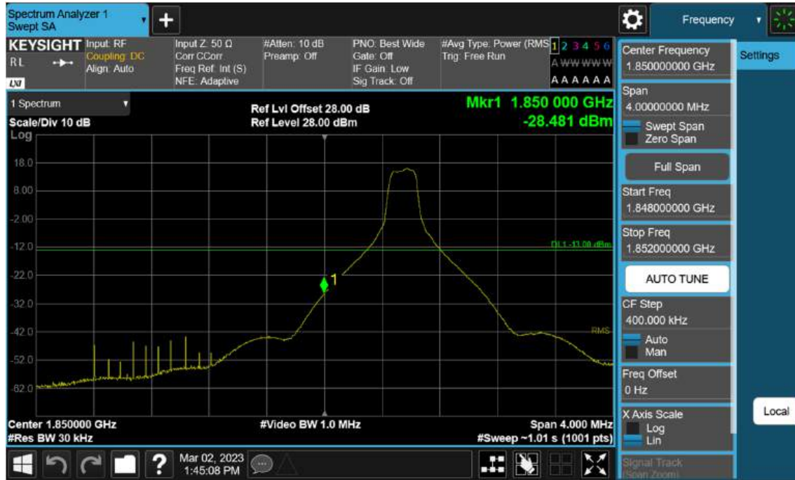
Sub6 n2. Lower Band Edge Plot (20 M BW Ch.372000 BPSK_RB1_Offset 0) -1
