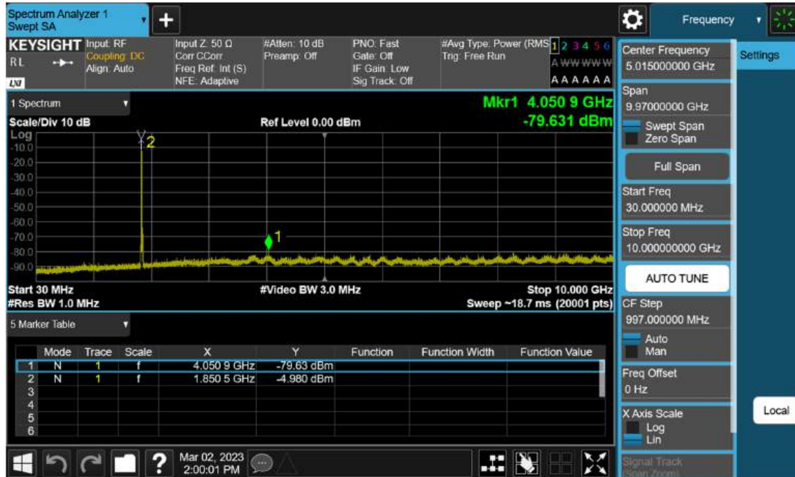
Sub6 n2. Conducted Spurious_1 (371500ch_15 MHz_ BPSK_RB 1_1)
