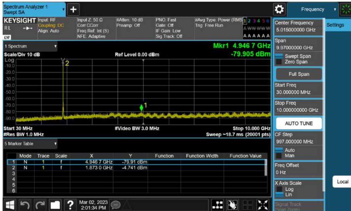
Sub6 n2. Conducted Spurious_1 (376000ch_15 MHz_ BPSK_RB 1_1)
