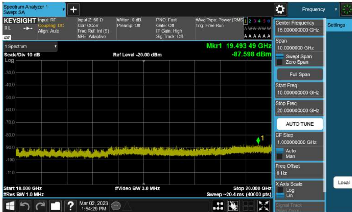
Sub6 n2. Conducted Spurious_2 (381500ch_5 MHz_ BPSK_RB 1_1)
