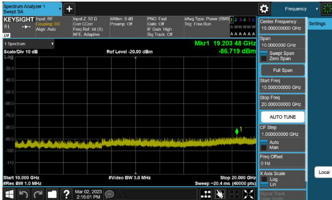
Sub6 n2. Conducted Spurious_2 (380000ch_20 MHz_BPSK_RB 1_1)
