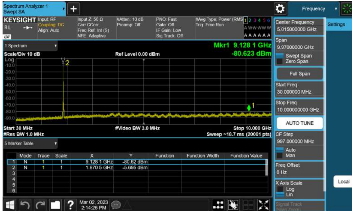
Sub6 n2. Conducted Spurious_1 (376000ch_20 MHz_ BPSK_RB 1_1)
