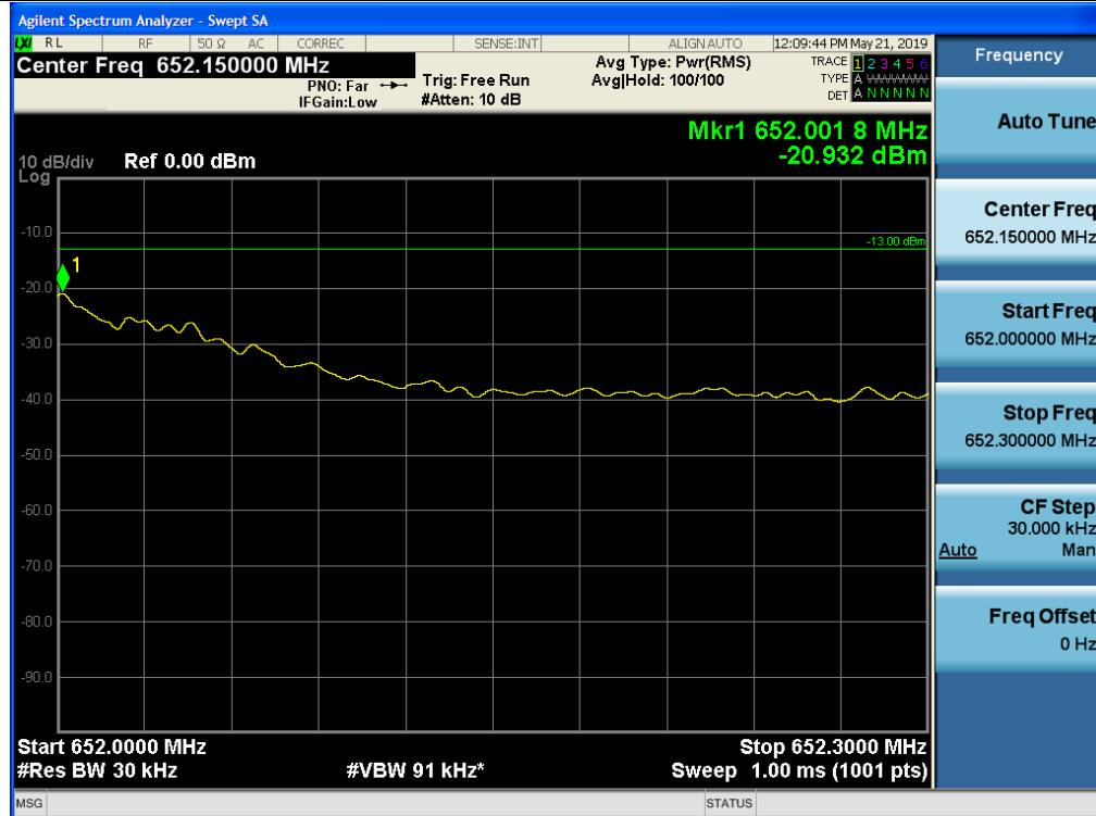
+3 dB above Out-of-band (two adjacent test signals) / 600 MHz Service / Downlink / LTE 5 MHz / Lower
