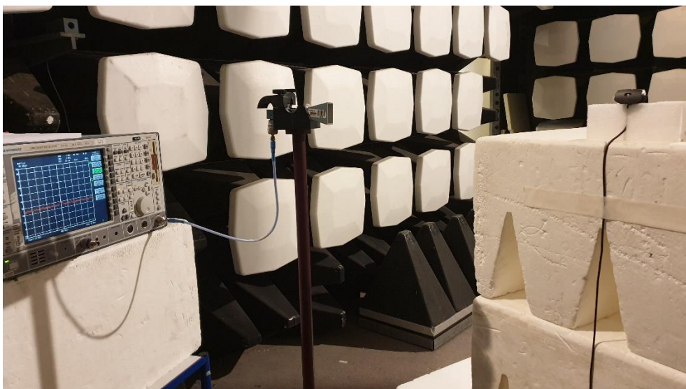
Photo 9. Radiated emission test setup for 14 - 25 GHz.
