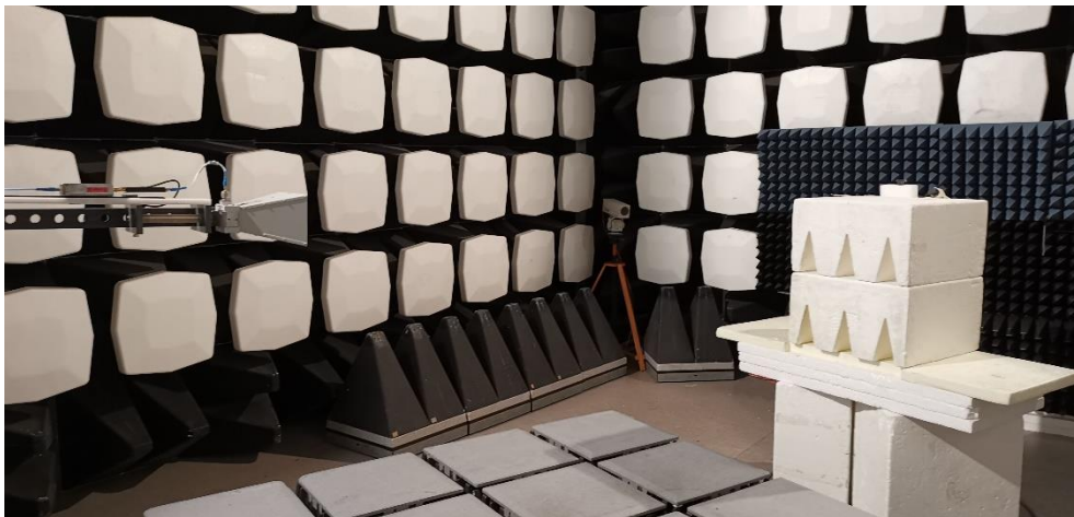
Photo 8 - Radiated emission test setup for 1 - 14 GHz.
