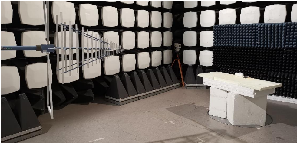
Photo 7 - Radiated emission test setup for 30 - 1000 MHz.
