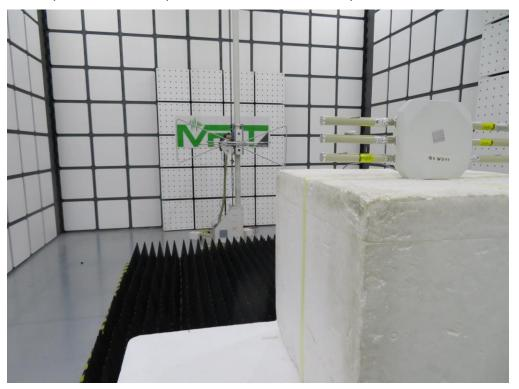
Description: Radiated Spurious Emissions Test Setup for above 1GHz\_AP361e
