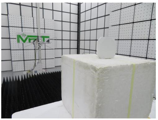
Description: Radiated Spurious Emissions Test Setup for above 1GHz\_AP361
