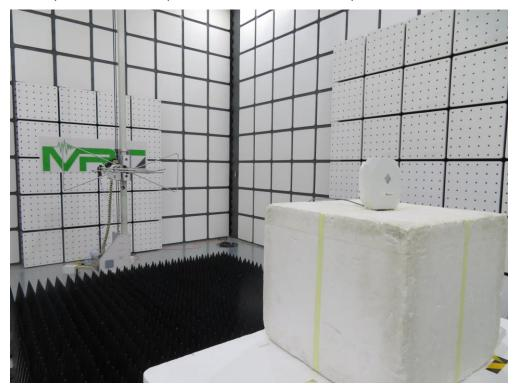
Description: Radiated Spurious Emissions Test Setup for above 1GHz\_AP361D
