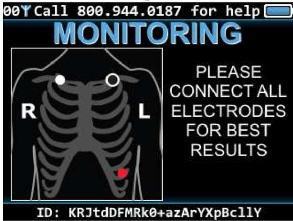
*An electrode has been disconnected.*
