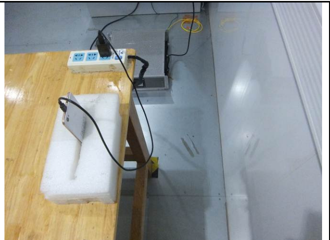
Conducted Emissions Test Setup Side View
