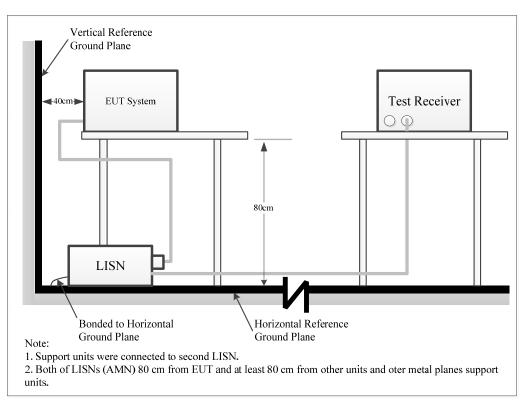
The setup of EUT is according with per ANSI C63.10-2013 measurement procedure. The specification used was with the FCC Part 15.207 limits.
