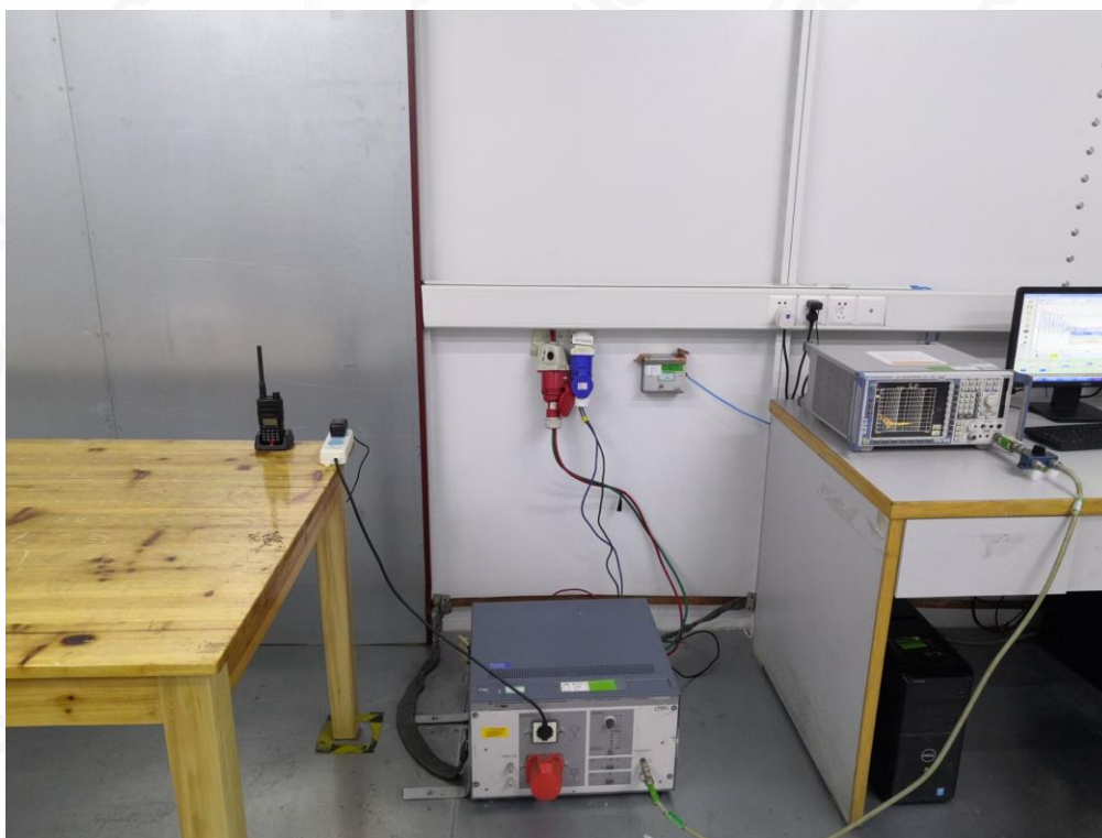
RADIATED EMISSION TEST SETUP-BELOW 1GHZ
