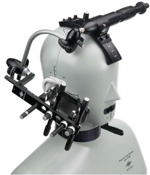
Figure 4-3 Heat and Torso Simulator (with Handset Positioner)
