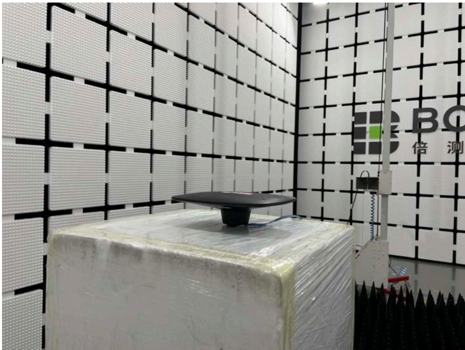
Spurious Emission Test Setup (Above 1GHz)
