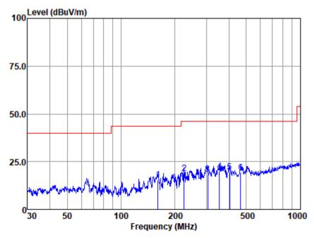
Antenna Polarity :VERTICAL EUT/Project :6155CR
