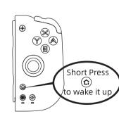
♦ After automatic sleep or manual shutdown, short pressing the @ will awaken the controller or reconnect to the previously paired device
