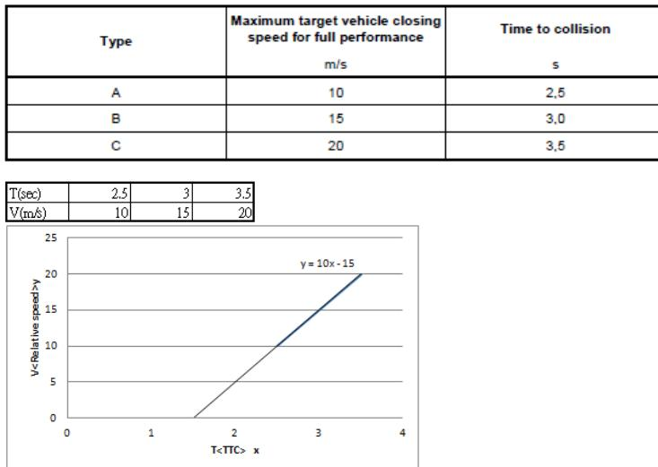
$$T = 0.1V + 1.5 \text{ (where } T \text{ is TTC and } V \text{ is relative speed)}$$
