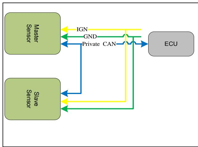
ECU is built by customer. The communication interface between 2 sensors is CAN (Private CAN or sensor CAN). The information on this CAN is vehicle data, sensor position setup data, warning parameter setup data and normal warning data output.
