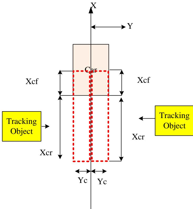
Position of Tracking Object will fall into the potential collision Region (length is Xcf+Xcr, Width is Yc for each side) with TTC within 2sec
