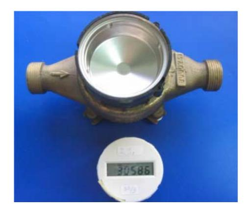
Photograph No.6 ETMW- LCD water reader extracted from external enclosure
