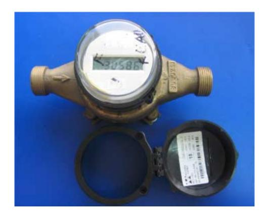
Photograph No.5 ETMW- LCD water reader extracted from external enclosure
