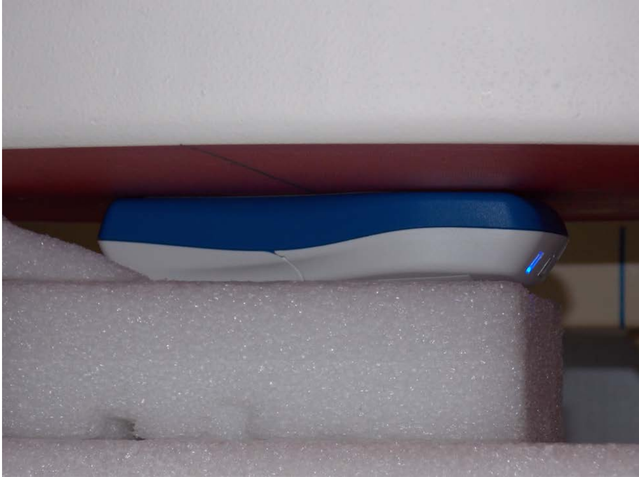
Test Position Back Face 10 mm Gap
