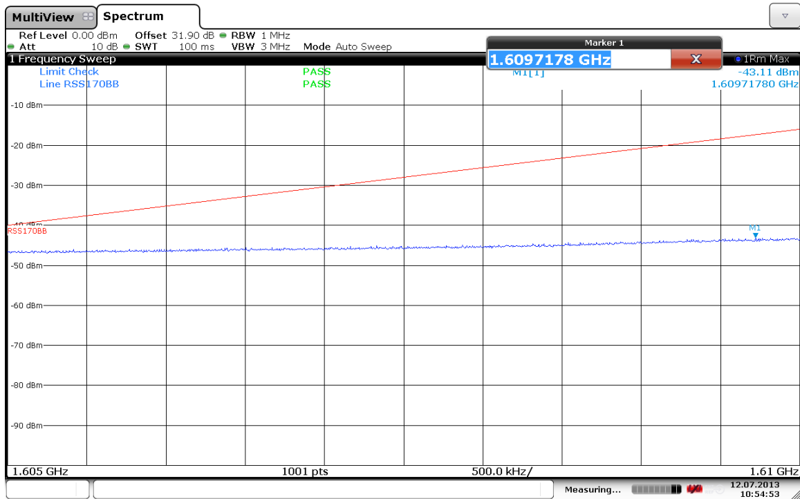
Additional Unwanted BB Emissions, r5t2x/r20t2x, 1626.6 MHz
