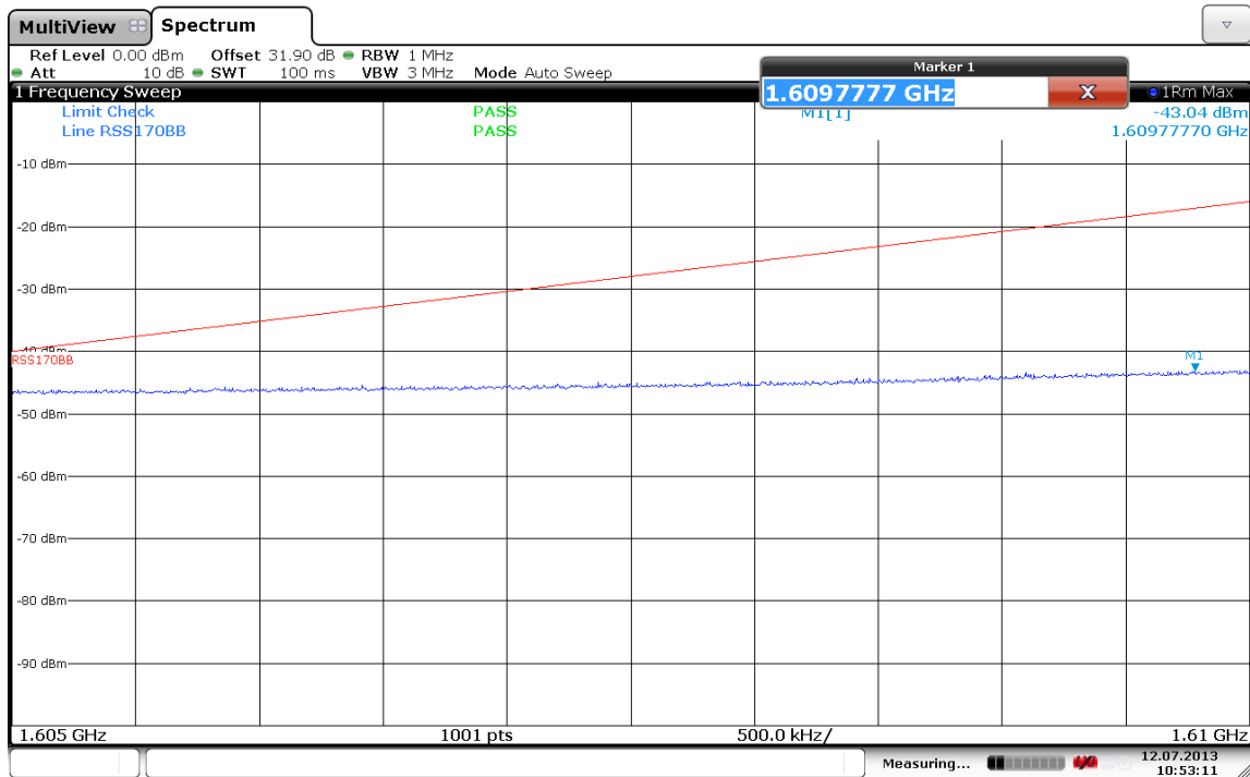
Additional Unwanted BB Emissions, r5t1x/r20t1x, 1626.6 MHz
