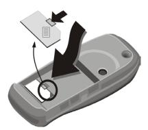
• Insert the battery sideways into the phone , then press downwards until it engages.
