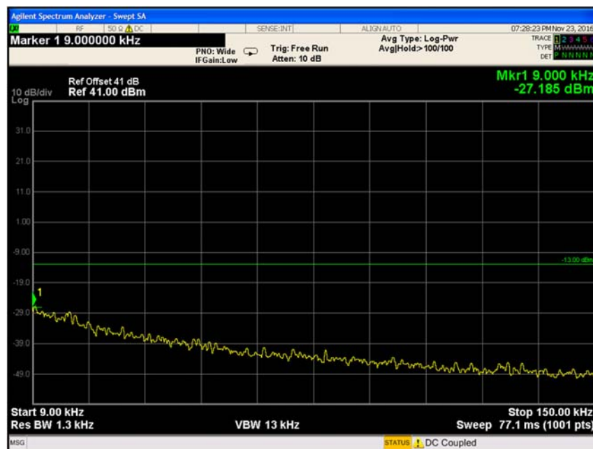
Figure 43 Spurious Emissions at Antenna Terminals 64QAM, 747MHz
