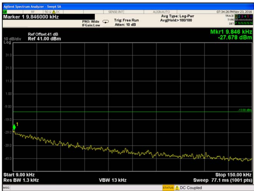
Figure 49 Spurious Emissions at Antenna Terminals QPSK, 733MHz
