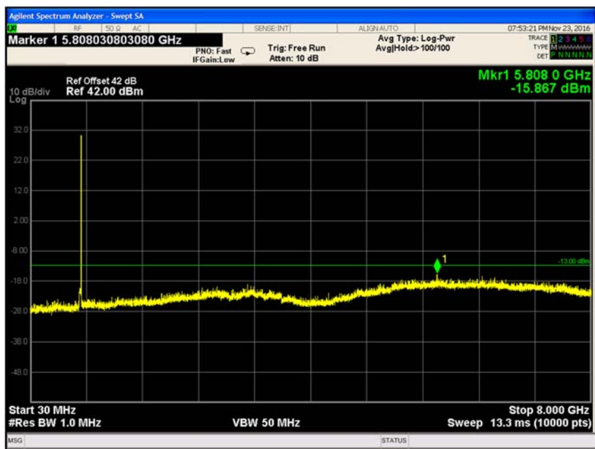
Figure 66 Spurious Emissions at Antenna Terminals 16QAM, 753MHz
