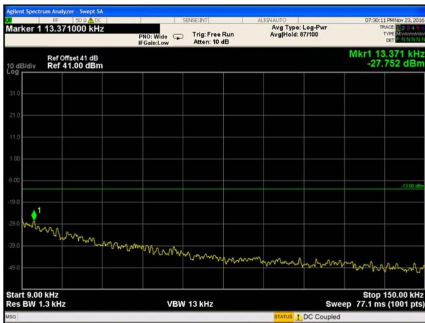
Figure 40 Spurious Emissions at Antenna Terminals 64QAM, 733MHz
