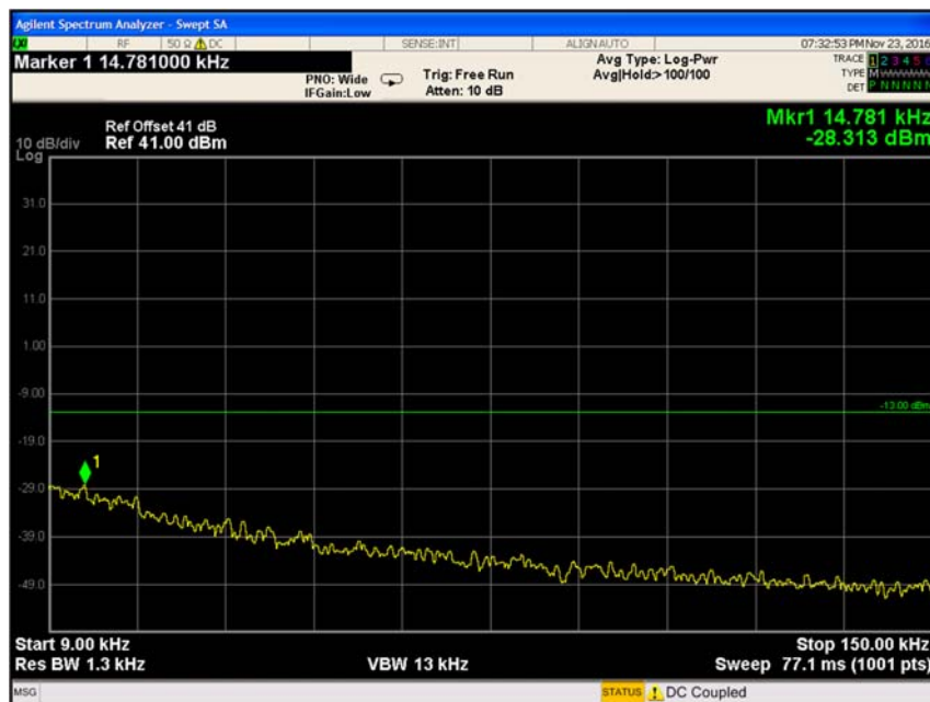
Figure 61 Spurious Emissions at Antenna Terminals 16QAM, 747MHz
