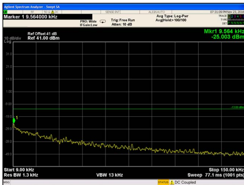
Figure 46 Spurious Emissions at Antenna Terminals 64QAM, 753MHz
