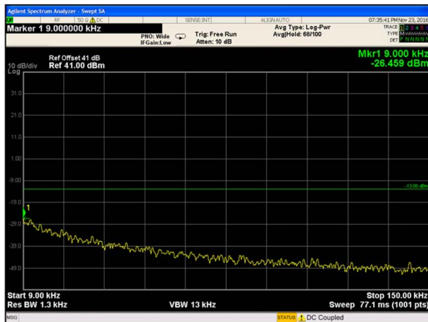
Figure 55 Spurious Emissions at Antenna Terminals QPSK, 753MHz
