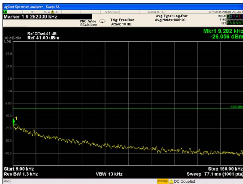
Figure 58 Spurious Emissions at Antenna Terminals 16QAM, 733MHz
