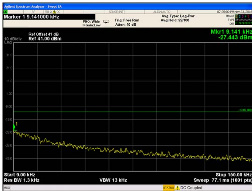
Figure 52 Spurious Emissions at Antenna Terminals QPSK, 747MHz
