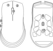
2.1. Key Description 1.Left click 2. Right click 3.Middle key (scroll key) Forward key Backward key 6.DPI 1).Six level DPI key: default DPI: 800 [ green ]. (DPI values can be customized and adjusted in the driver software DPI indicator light: 400 (Red) | 800 (Green) | 1200 (Blue) | 1600 (Blue) | 2400 (Yellow) | 3200 (Purple)
