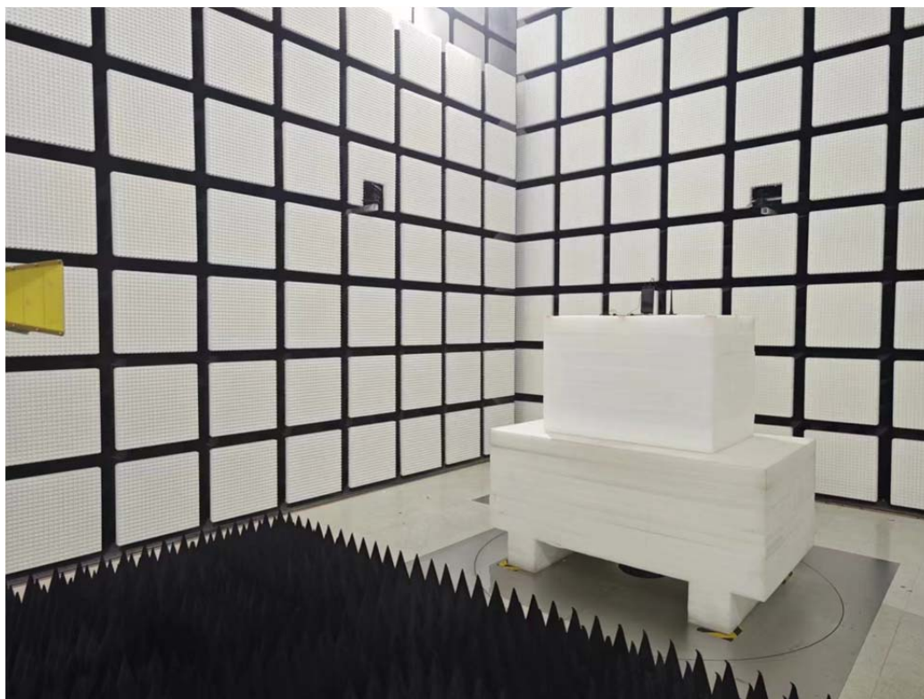
Radiated Emission 1-18GHz View
