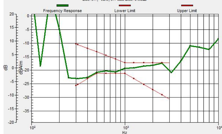
General Scans_LTE band5_T-Coil_HAC 3/z (axial) wideband at best S/N/ABM Freq Resp(x,y,z,f) Loc: 3.7, -12.3, 3.7 mm Diff: 0.18dB
