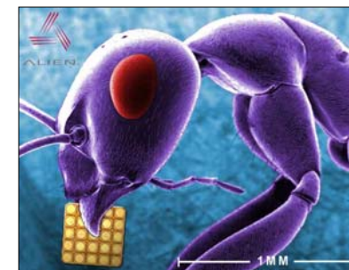
Ant with Alien 350 micron NanoBlock™ IC.
