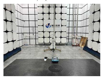
Test frequency from 30MHz to 1GHz
