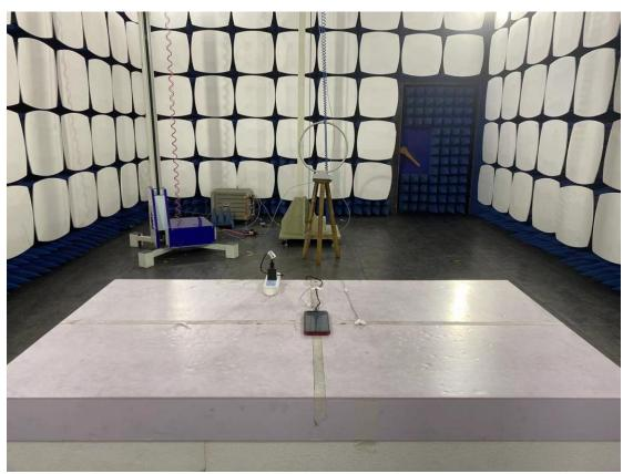
3. Radiated emission (9KHz-30MHz)
