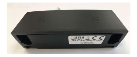
FCC and IC ID of the module is located under the module and can be read when reader is fixed in a wall
