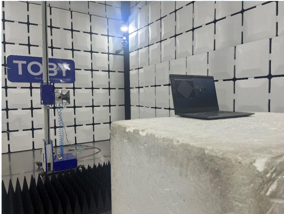
Photo of Setup for Conducted Emission
