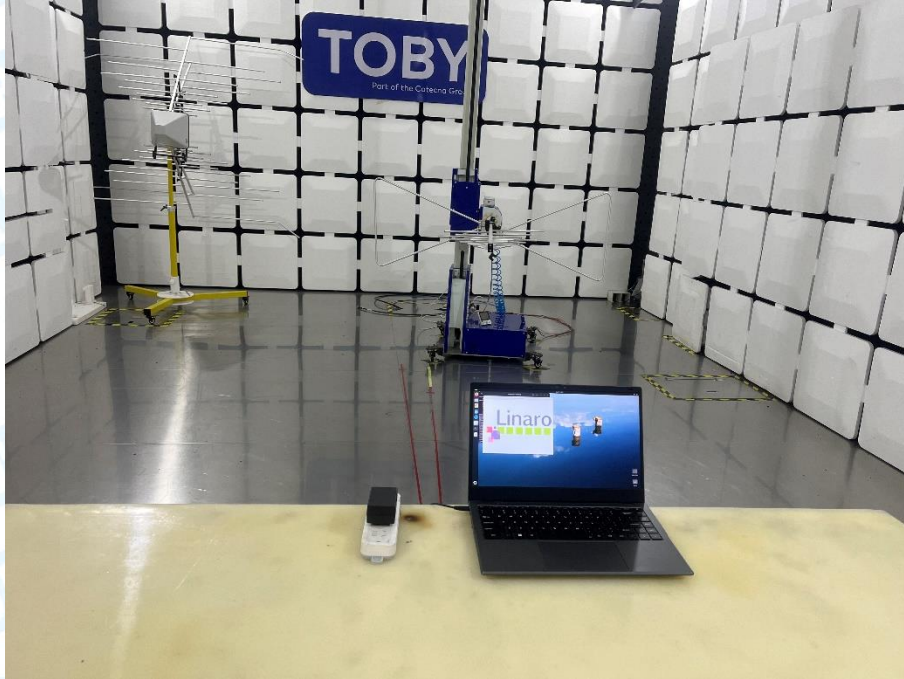
Photo of Setup for Radiated Emission (Below 1 GHz) ----GENBOOK-RK3588-X0
