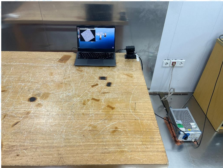
Photo of Setup for Conducted Emission
