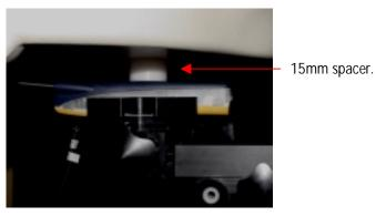
Note: the 15mm spacer was removed during the SAR measurement.
