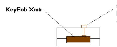
Test tool with screw to engage transmit button. Material: clear plastic.
