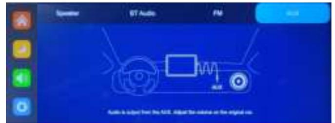
(4) [AUX]: After selecting this mode, the AUX output mode will be turned on. Connect the equipment to your vehicle's AUX port with an AUX cable. After the connection is successful, set your car to be AUX-IN mode, then all the sounds of the equipment will be transmitted to your vehicle speakers through the AUX cable.
