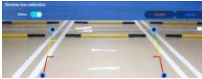
Park your car in the middle of the parking zone, manually hold and drag
