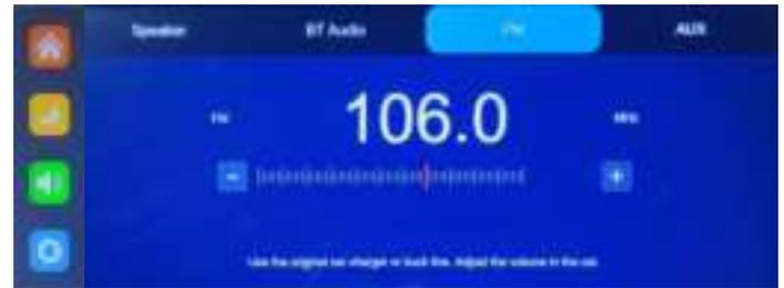
(3)[FM]: After selecting this mode, FM transmission mode will be turned on. For example, the FM transmitting frequency band of this equipment is set to FM106.0MHz(any unoccupied channel can be used), tune your car radio to the same frequency FM 106.0 MHz, then all sounds of the equipment will be transmitted to your vehicle radio.
