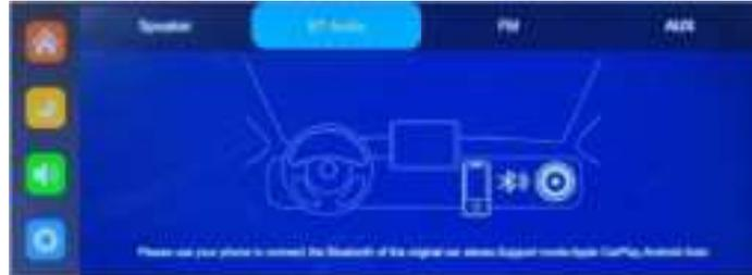
(2) [Bluetooth]: After selecting this mode [BT Audio], the Bluetooth transmission mode will be returned on. Turn on your vehicle's Bluetooth then, connect your cell phone's Bluetooth to your car. After the car Bluetooth connection is successful, all the sounds of the device will be transmitted to your car speakers through Bluetooth transmission.
